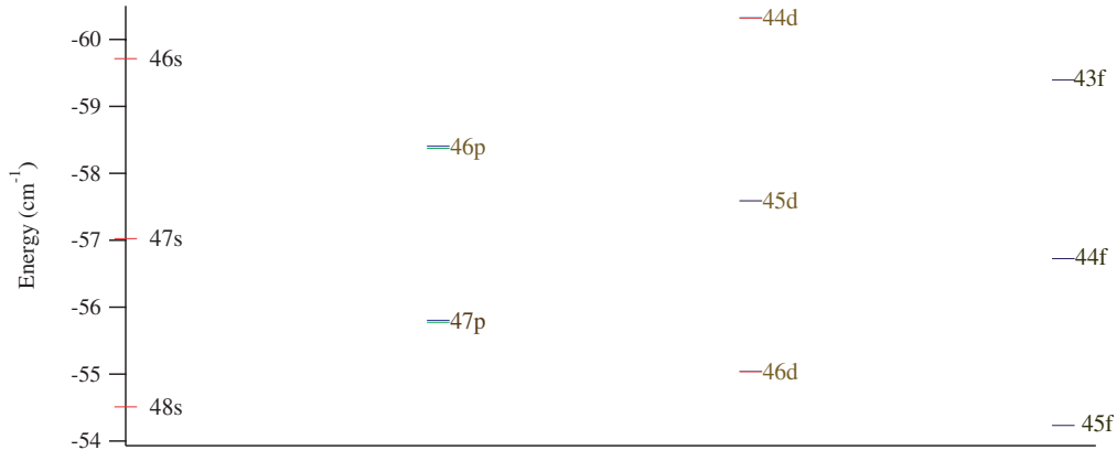
Fig. 7.2: Energy level spacing near n=47 Rydberg states. Pairs of atoms can be nearly degenerate with atoms in nearby states, resulting in large Van der Waals interactions.
