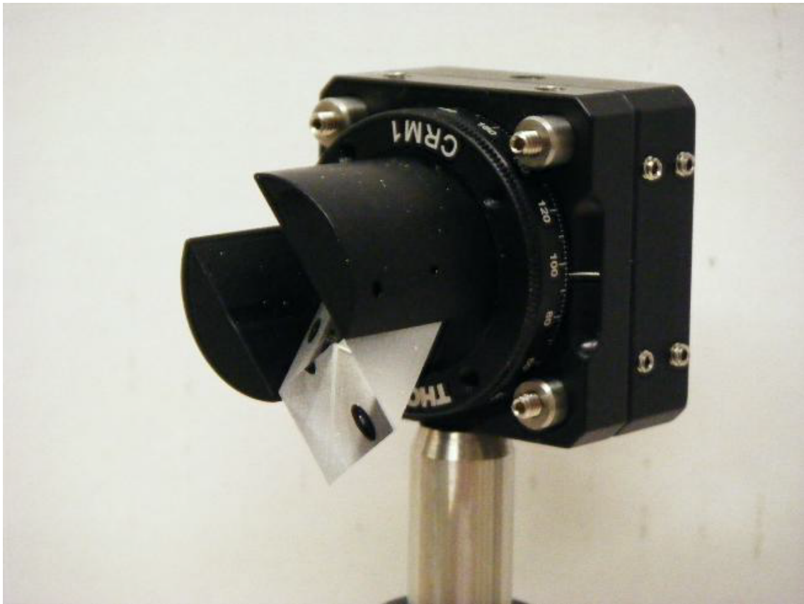
Figure D.3 Input side of Fresnel-Rhomb and polarizing beam splitter setup.
