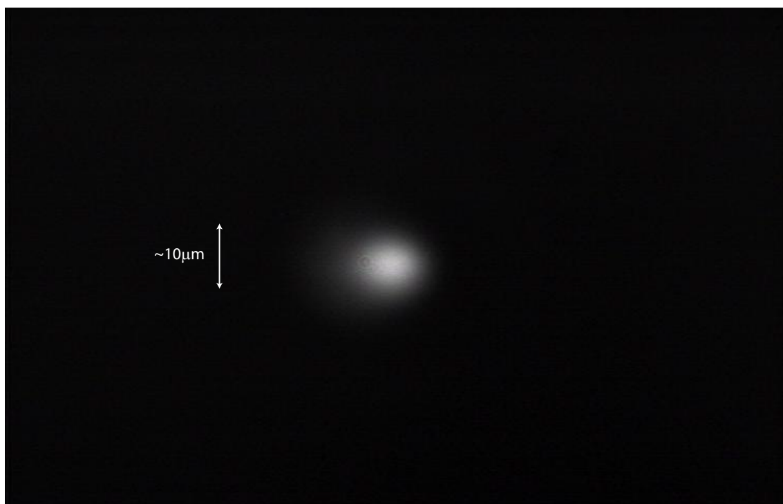
Figure E.3 Image showing the FORT side 780nm addressing laser beam prior to installing the AOM.
