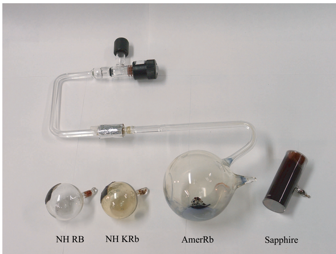
Fig. 3.5: Picture of several of the HySEOP cells used in this work. The slight discoloration of the NH KRb cell due to reactions with high temperature K can be seen in comparison with the NH Rb cell. The body of the Sapphire cells shows the discoloration of glass due to Na after less than 1 week.
