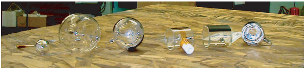
Figure 5.2: Picture showing some of the Rb- ^3\text{He} cells used to measure spin-exchange rate coefficients.
